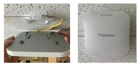
Ensure the Sensor is securely latched in place. The mounting is complete.
